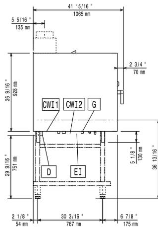
CWI1 = Raccordement eau froide      G = Connexion gaz
